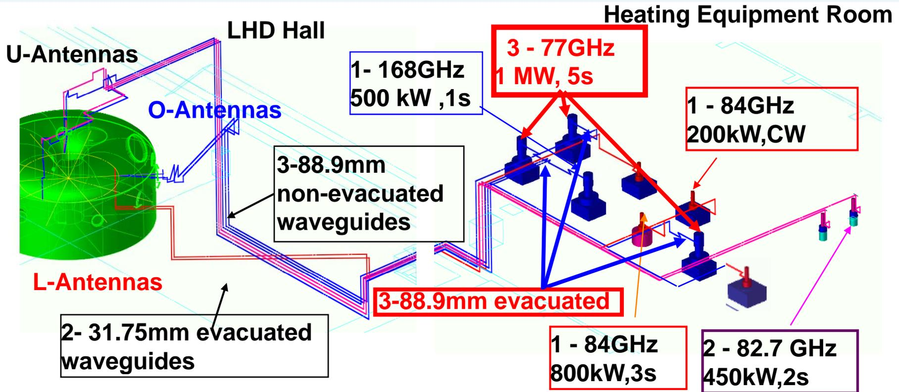
9 gyrotrons, transmission Lines, antennas are operated.
