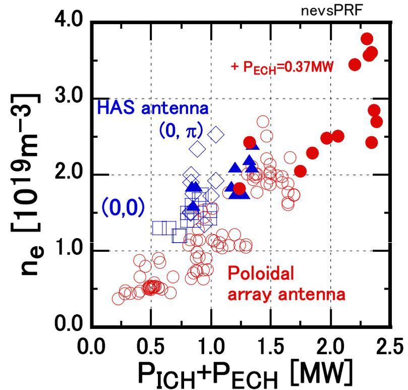
By using four antennas (a pair poloidal array antenna, a pair of HAS antenna),  $n_e$  of  $3.7 \times 10^{19} m^{-3}$  and  $T_i \sim T_e \sim 1$  keV is stably sustained. Pulse length can be elongated in this experimental campaign.
